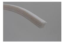
**4002 PTFE WITH SILICON RUBBER CORE PACKING**MK4002 is braided with 4000Y and blended with silicone rubber in central position. It has excellent compensation performance and is applicable for valves, vessels and pumps of corrosive media in chemical, medicine, food, petrochemical and power industry.
